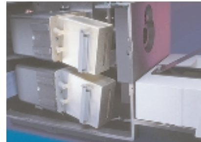
Dual-beam design features two spectral analyzers for superior stability and greater productivity.
